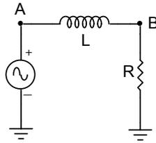
$$V_s = V_L + V_R \Rightarrow V_0 \sin(\omega t) = L \frac{di}{dt} + R i \quad (6.4)$$
